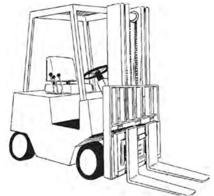
Figure 22. Counterbalance Lift Truck
